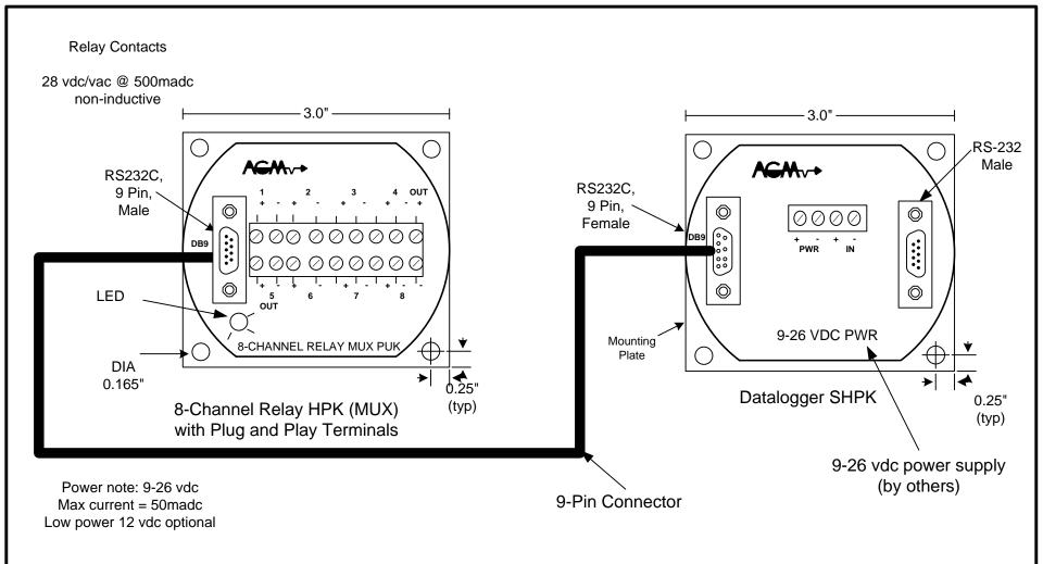
NOTE: Use "AGM Datalogger Disk" for SHPK Configurations and Data Download. Sub-assemblies Suitable for bulkhead mounting (Vertical or Horizontal)
