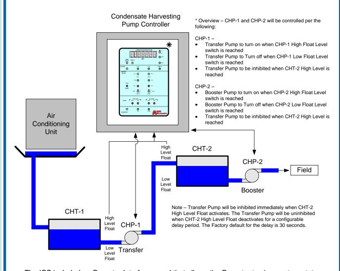
The ICS included an Operator Interface panel that allows the Operator to view system status as well as manually operate the pumps and adjust system parameters such as pump on-off delay timers.
